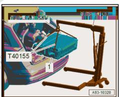
Pry out the high-voltage battery -1- from the vehicle using the -VAS6100- .
