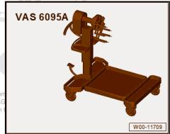
Engine/Transmission Holder - Universal Mounting - VAS6095/1- and Engine and Transmission Holder - Bracket (V6 TDI Engine) - VAS6095/1-14-
