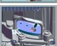
To loosen the bolts for the torsion dampers, counterhold the crankshaft using the -T40263- and -T40314- .
