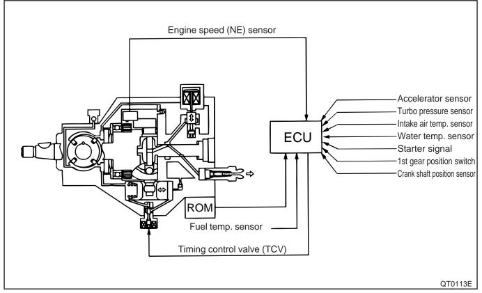
As with the ECD-V3 (ROM), the ECD-V4 determines the duty ratio by comparing the target and actual injection timings.
