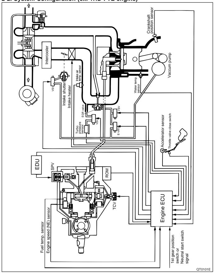
2-2. System Configuration (ex. 1HD-FTE engine)
