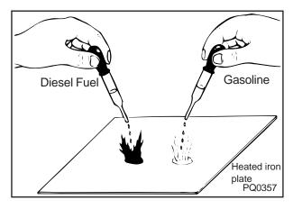
The measurement that is used to indicate the ignitability of diesel fuel is the cetane value. A fuel with a low cetane value has poor ignitability and a longer ignition lag time, which leads to diesel knocks.
