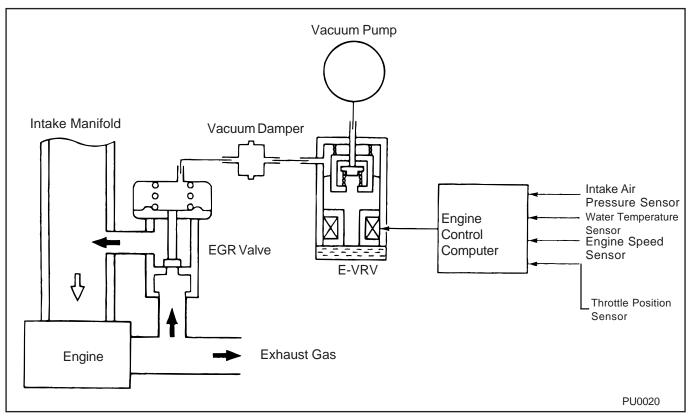
Based on the acceleration opening (throttle position sensor), engine speed, coolant water temperature, intake air pressure, and intake air temperature signals, the computer determines the volume of the recirculation of the exhaust gases and effects duty-cycle control in the operation of the vacuum control valve (E-VRV).
