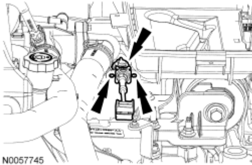
Fig. 371: Identifying RH Camshafts Bolts Courtesy of FORD MOTOR CO.
