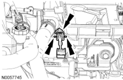
Fig. 352: Aligning Timing Marks On Variable Camshaft Timing (VCT) Assemblies Courtesy of FORD MOTOR CO.
