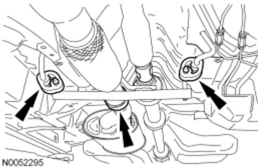
Fig. 874: Locating Subframe Support Brackets And Bolts Courtesy of FORD MOTOR CO.
