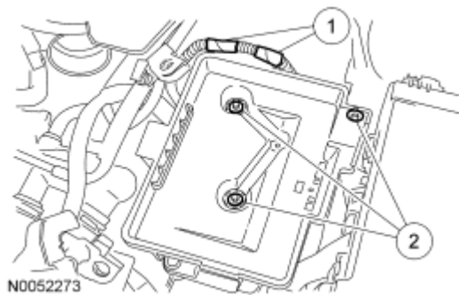
Fig. 292: Locating Push Pin Fasteners & Front Splash Shield Screws Courtesy of FORD MOTOR CO.
