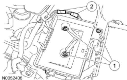
Fig. 691: Locating Power Steering Pump Bolts Courtesy of FORD MOTOR CO.
