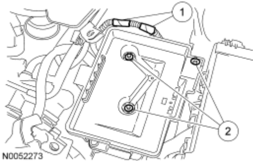
Fig. 678: Locating Engine Lifting Eye & Bolts Courtesy of FORD MOTOR CO.
