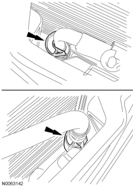
Fig. 284: Identifying Fuel Hose Routing Clip From Transaxle Stud Courtesy of FORD MOTOR CO.
