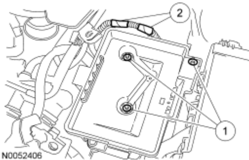
Fig. 960: Locating LH Exhaust Manifold Studs Courtesy of FORD MOTOR CO.
