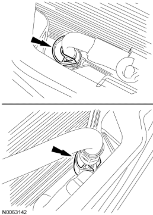
Fig. 294: Disconnecting Transmission Cooling Tubes Using Special Tool (307-569) Courtesy of FORD MOTOR CO.
