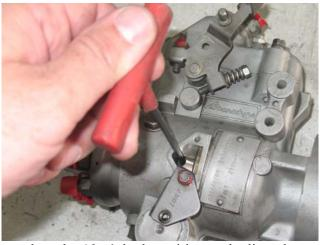
Insert and allen wrench at the 12 o'clock position and adjust the screw clockwise the increase fuel delivery. For every 1/8 of a turn you should increase delivery 5-7% DO NOT adjust more that a ½ turn without checking drivability of the engine.
