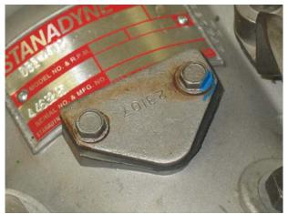
Remove the two screws that hold the plate to the pump.
