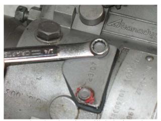
After removing the plate, fuel will drain from the pump.
