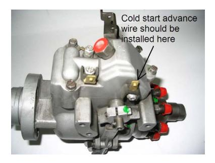
2) You should also have the pump properly timed. Please refer to the manufacturers timing information for complete timing instructions. Most 6.9 and 7.3L applications, when properly timed, have the timing mark advanced (toward the drivers side of the vehicle) approximately 1/8 inch off the engine timing mark.
