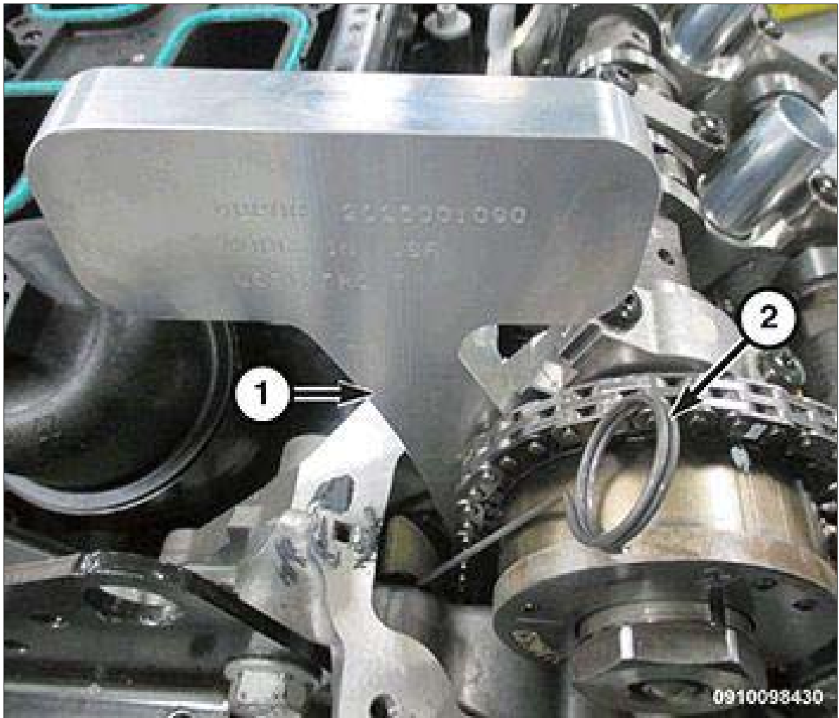
Fig 9: Holding Pawl Off Rack & Pushing Timing Chain Tensioner Holder Into Place
