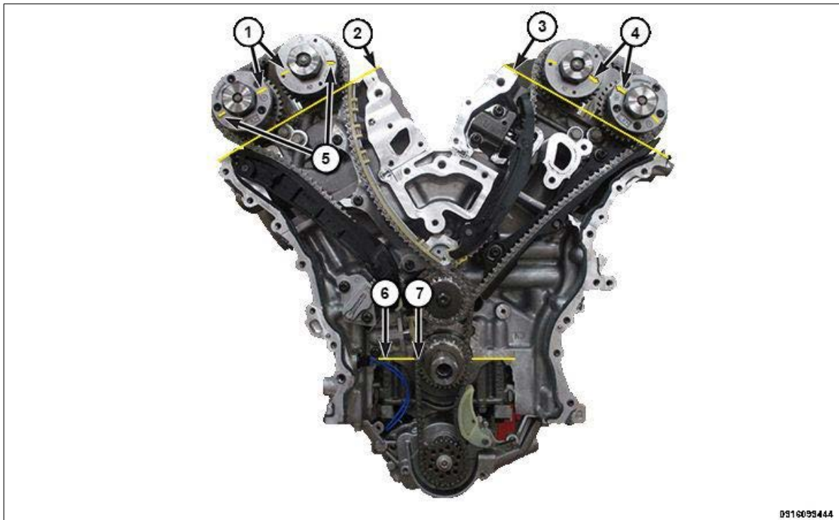
Fig 7: Scribe Lines, Valve Cover Sealing Surfaces, Cam Phaser Arrows, Block/Bearing Cap Junction & Dimple
