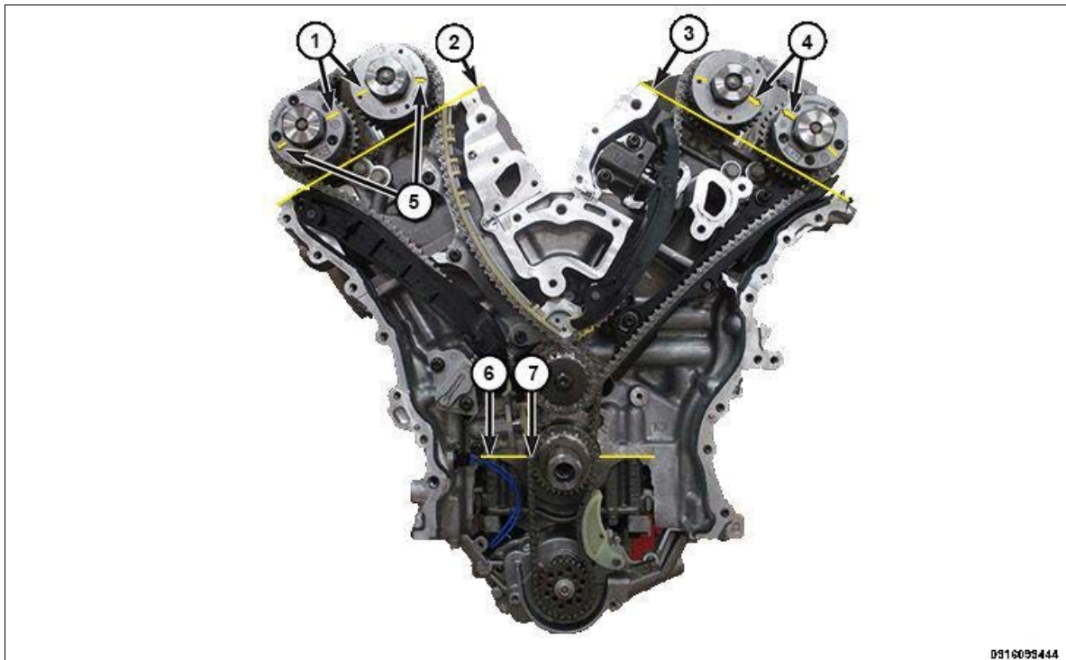
Fig 6: Scribe Lines, Valve Cover Sealing Surfaces, Cam Phaser Arrows, Block/Bearing Cap Junction & Dimple
