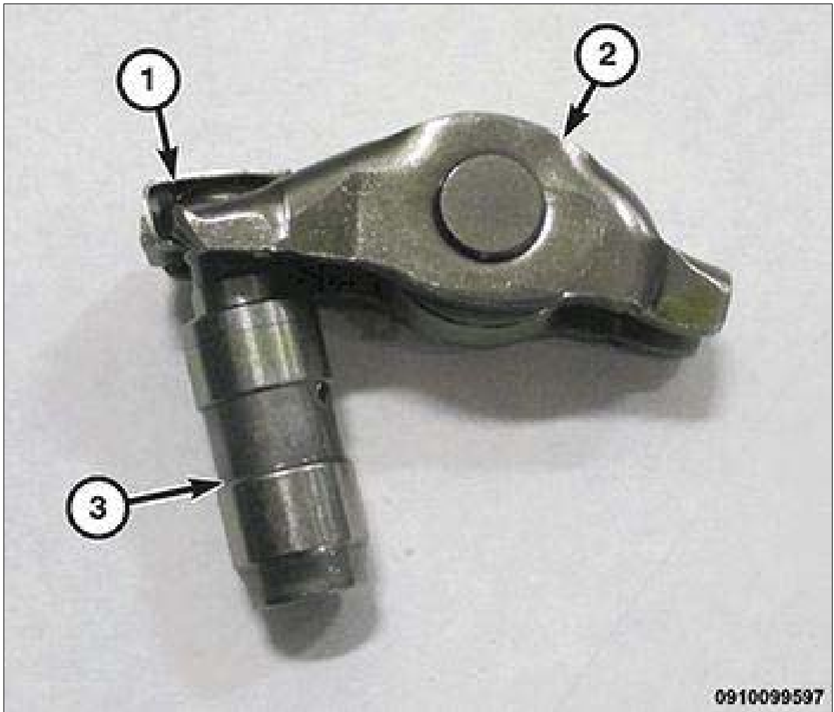
Fig 2: Retaining Clip, Exhaust Roller Rocker Arms & Hydraulic Lifters
