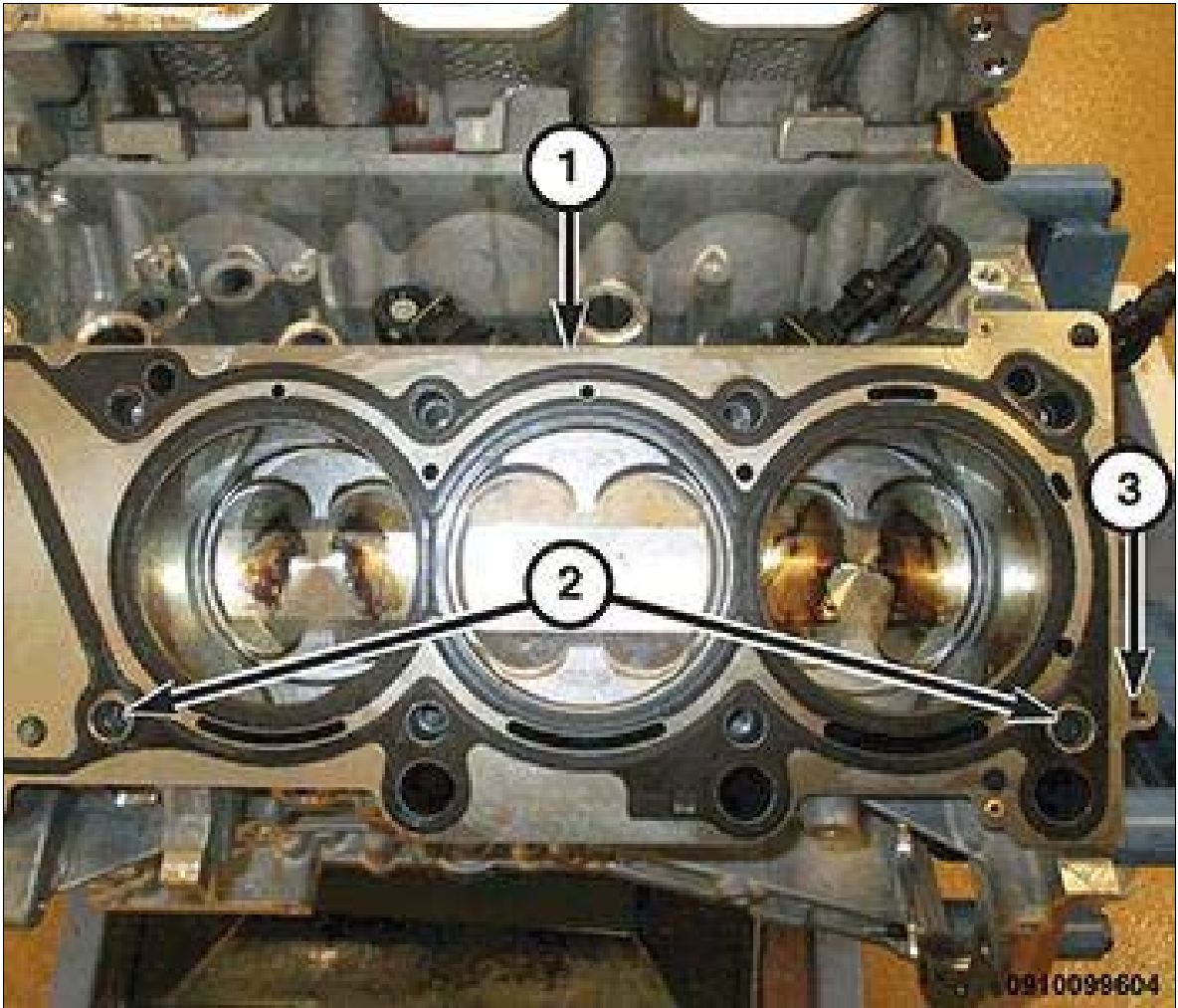
Fig 7: Head Gasket, Locating Dowels & Identifying Mark
