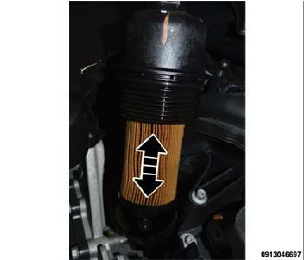
Fig 3: Remove/Install Oil Filter From/To Housing
