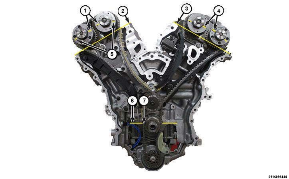
Fig 1: Scribe Lines, Valve Cover Sealing Surfaces, Cam Phaser Arrows, Block/Bearing Cap Junction & Dimple
