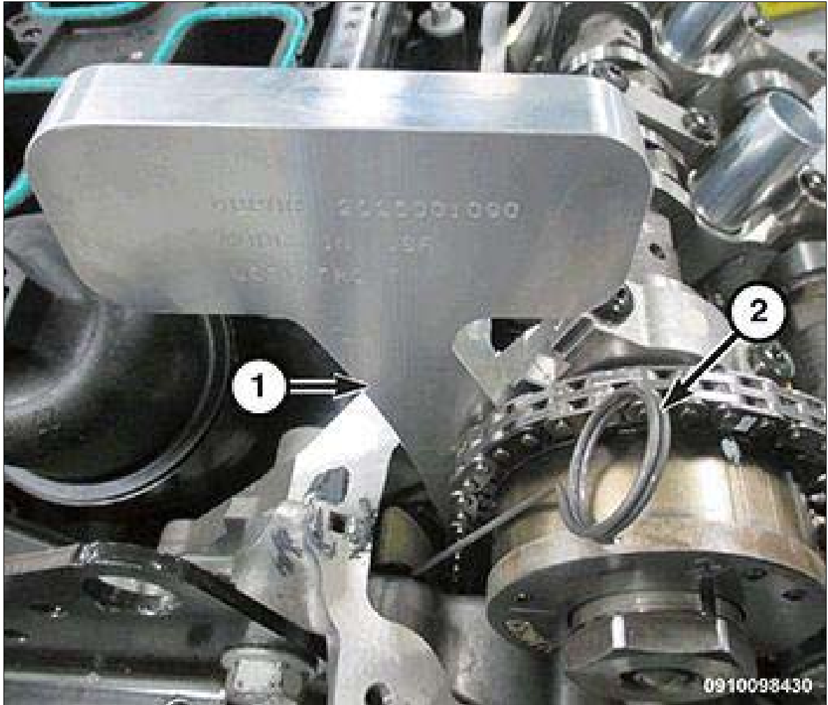
Fig 2: Holding Pawl Off Rack & Pushing Timing Chain Tensioner Holder Into Place
