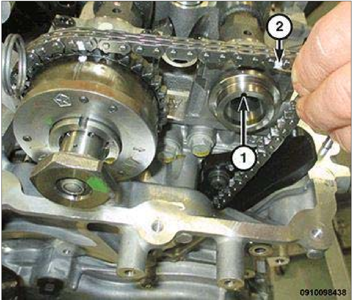
Fig 12: Exhaust Camshaft & Timing Chain
