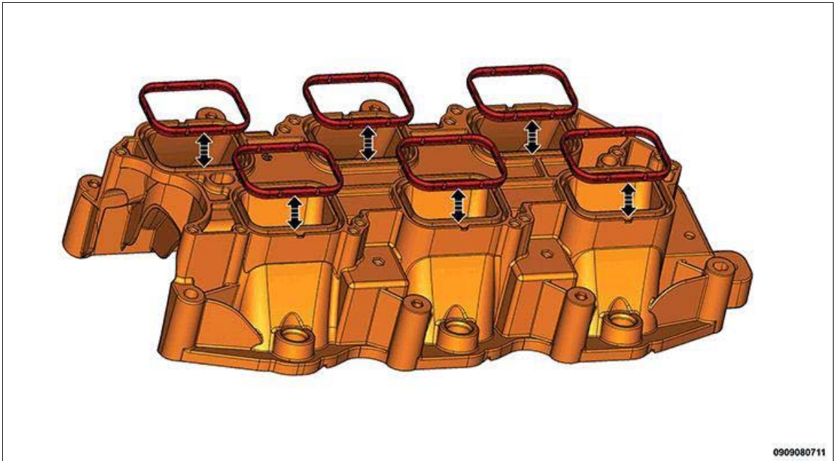
Fig 12: Upper To Lower Intake Manifold Gaskets
