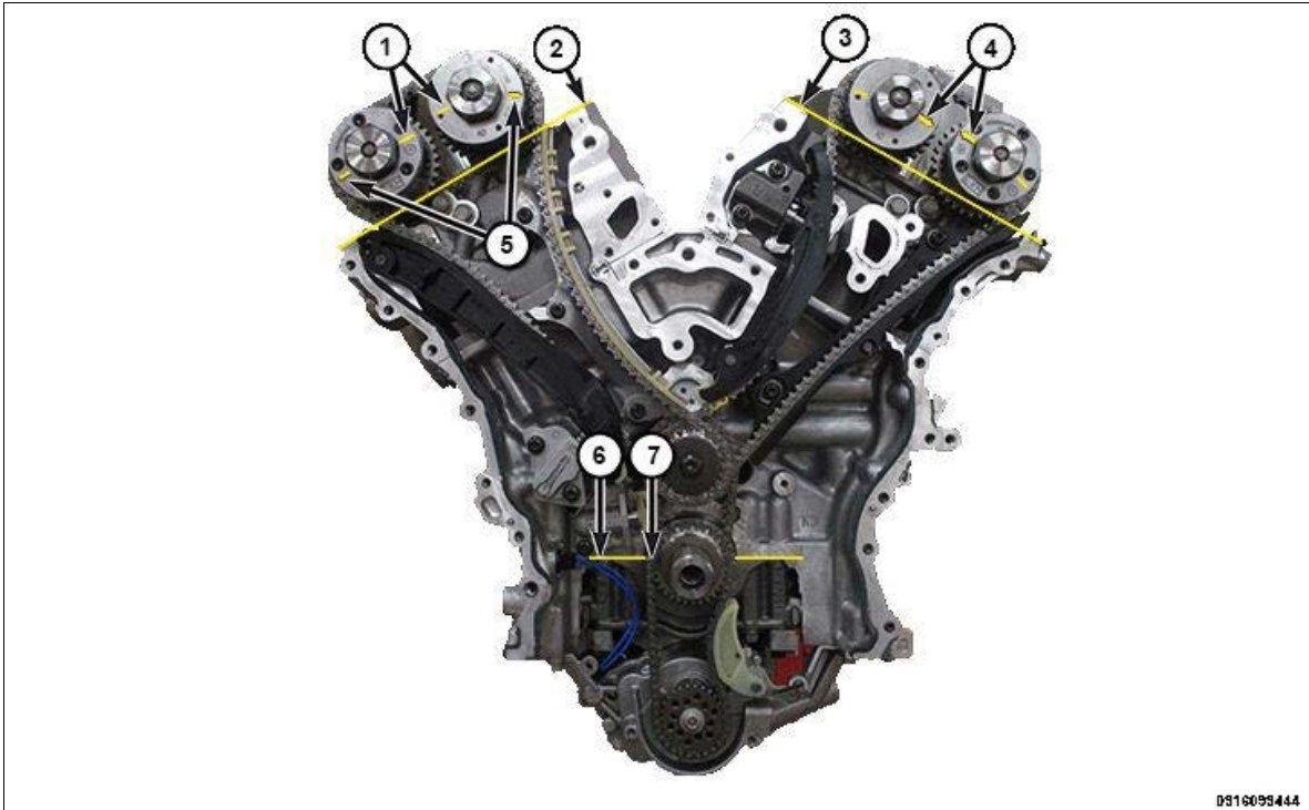
Fig 4: Scribe Lines, Valve Cover Sealing Surfaces, Cam Phaser Arrows, Block/Bearing Cap Junction & Dimple
