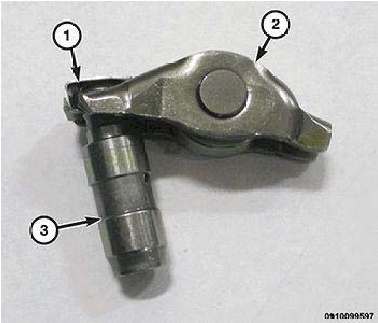
Fig 1: Retaining Clip, Exhaust Roller Rocker Arms & Hydraulic Lifters
