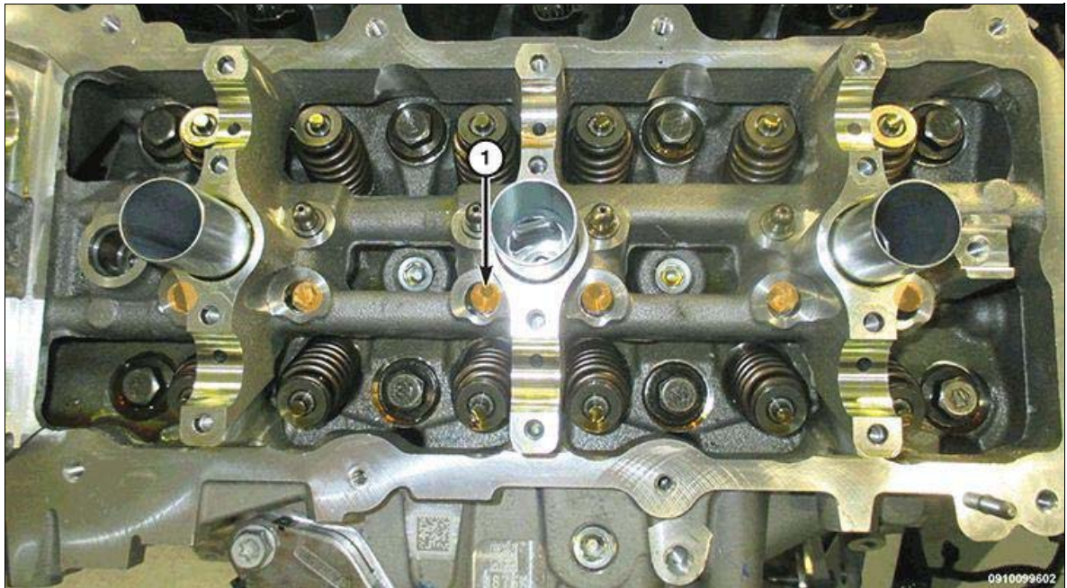
Fig 2: Locating Exhaust Hydraulic Lifters
