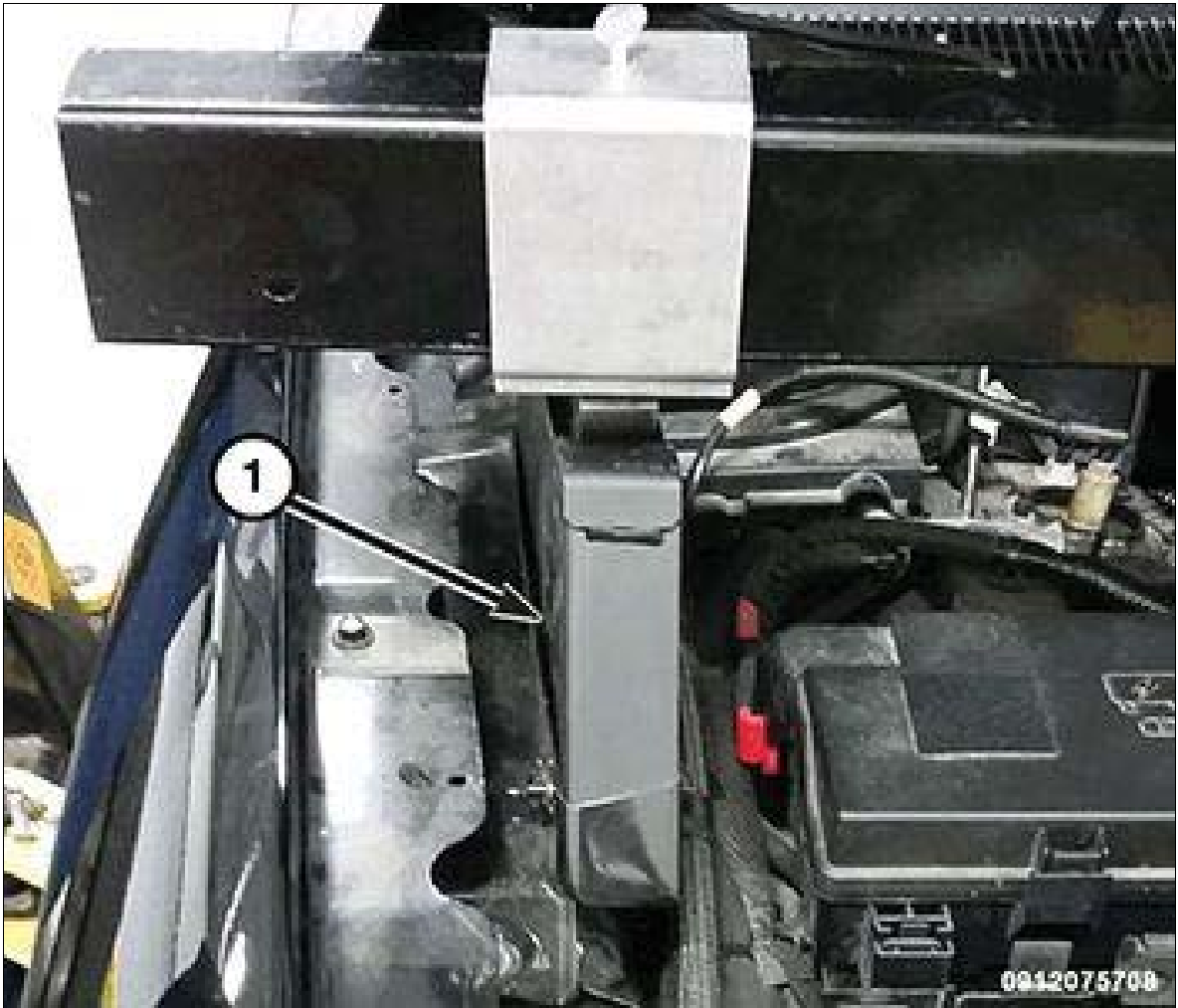
Fig 3: Placing Engine Support Fixture On Right Side Of Inner Body Structure
