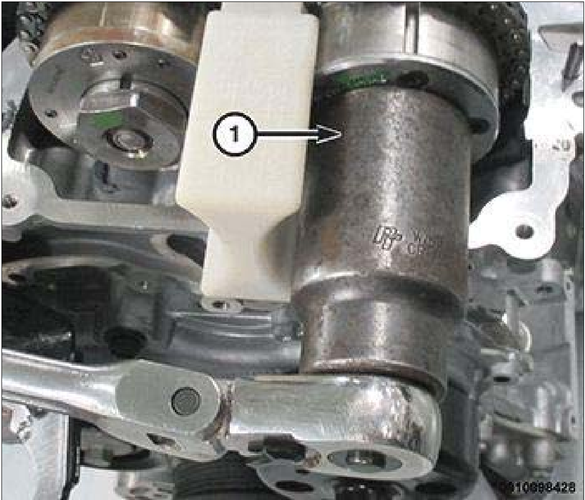
Fig 7: Installing Socket On Exhaust Oil Control Valve
