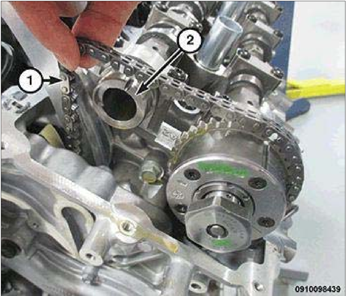
Fig 13: Intake Camshaft & Timing Chain
