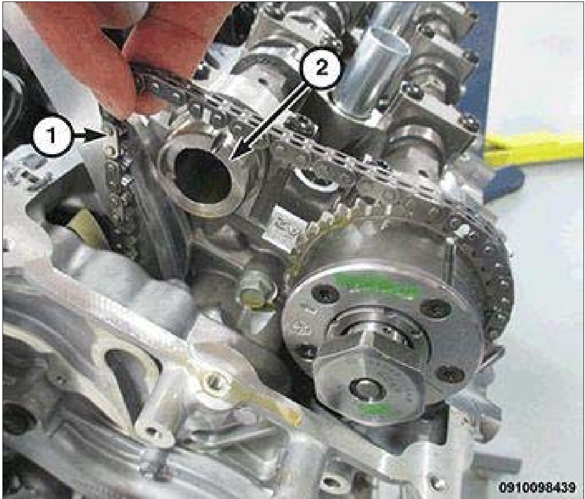
Fig 2: Intake Camshaft & Timing Chain
