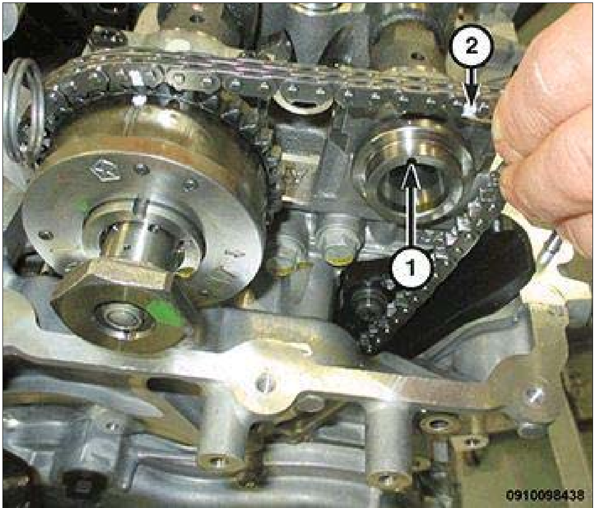
Fig 3: Exhaust Camshaft & Timing Chain
