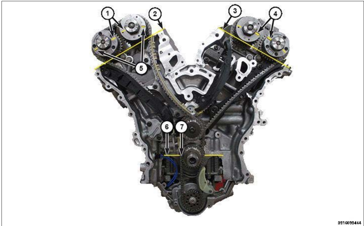
Fig 17: Scribe Lines, Valve Cover Sealing Surfaces, Cam Phaser Arrows, Block/Bearing Cap Junction & Dimple
