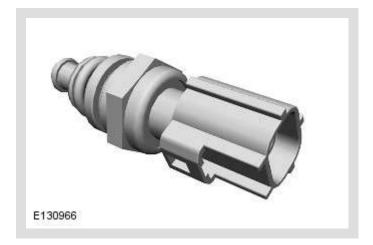
The ECT is located in the thermostat housing. The ECM uses the temperature information for the following functions:
