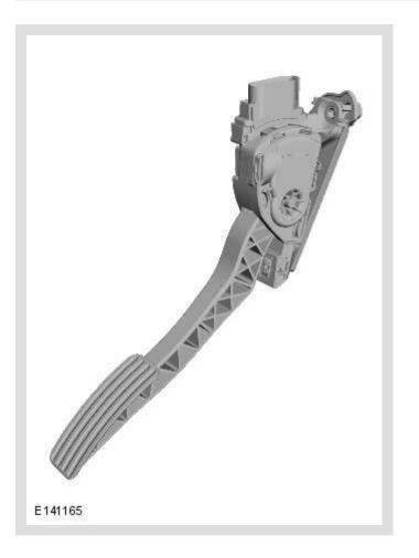
The APP sensor allows the ECM to determine the driver requests for vehicle speed, acceleration and deceleration. The ECM uses this information to determine the torque demand from the engine via injection control.
