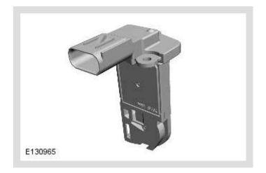
Identical MAFT sensors are installed in the air cleaner outlets, but only the MAFT sensor in the right air cleaner provides both MAF and temperature signals for the ECM . The engine harness connection with MAFT sensor attached of the left air cleaner is wired so that only the MAF signal is connected to the ECM .
