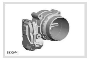
The electric throttle is installed at the front of the engine, between the cylinder heads. The throttle plate is operated by a DC (direct current) electric motor attached to the throttle body. The motor is controlled by the ECM , which operates the motor in response to driver inputs from the APP sensor and other engine related sensors to provide the correct air flow to the intake manifolds.
