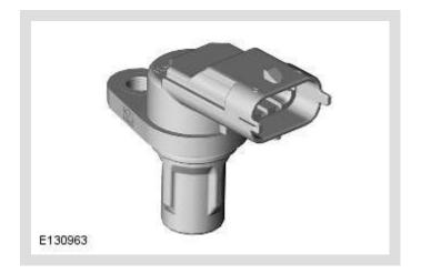
The CMP sensor is located on the rear face of the left cylinder head. The sensor tip protrudes through the face to pick up on the reluctor ring behind the camshaft pulley. The CMP sensor is a Hall effect type sensor.
