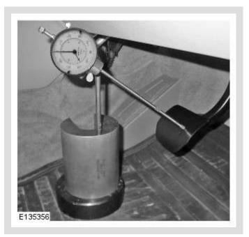
Position the DTI gauge on a suitable mounting block, as illustrated.
