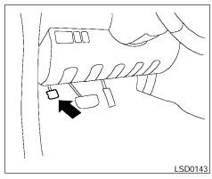
**To engage:** Firmly depress the parking brake.
