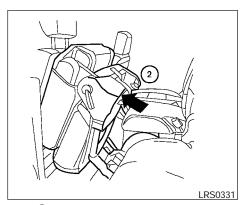
Then (2) lift up on the lower corner of the seat base and tip the outboard seating position of the 2nd row bench seat forward. To exit the 3rd row bench seat lift up on the same latch and fold the seatback forward onto the seat base. Then lift up on the seat base and tip it forward.
