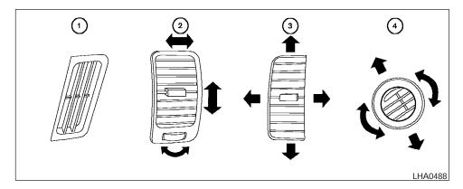
Adjust air flow direction for the driver and passenger side windows(1), driver and passenger front (2) center(3), rear passenger compartment (4) and rear center console (if so equipped) ventilators(5) by moving the ventilator slide and/or ventilator assemblies.
