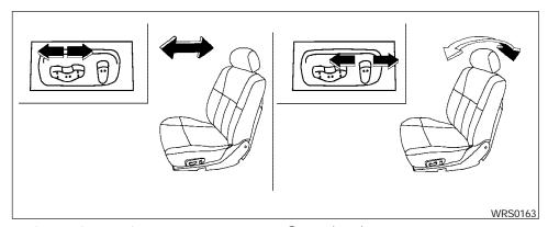
FRONT POWER SEAT ADJUSTMENT (if so equipped)
