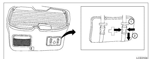
A first aid kit is located on the back door trim panel. To remove the first aid kit:
