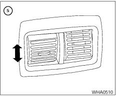
rear center console ventilators (if so equipped)
