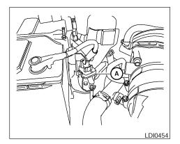
If you add electrical accessories to your vehicle ground it to the body ground (a) located near the battery along the negative battery cable.
