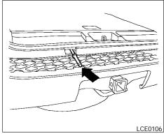
4. Find the oval-shaped opening above the middle of the bumper. Pass the T-shaped end of the jack rod through the opening and direct it toward the spare tire winch, located directly above the spare tire.
