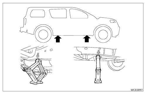
Place the jack directly under the jack-up point as illustrated so the top of the jack contacts the vehicle at the jack-up point. The jack-up points are indicated by stamped arrows on the side of the frame.
