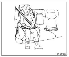
low back booster seat (1) is chosen, the vehicle seat back must be at or above the center of the child's ears. If the seat back is lower than the center of the child's ears, a high back booster seat (2) should be used.
