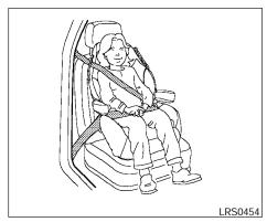
BOOSTER SEAT INSTALLATION ON FRONT PASSENGER SEAT
