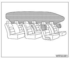
Supplemental side-impact air bag (if so equipped) and curtain side-impact and rollover air bags (if so equipped) system
