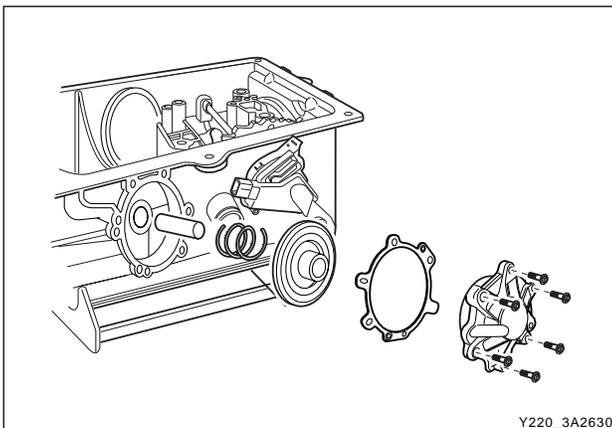
12. Remove the rear servo cover and piston assembly.
