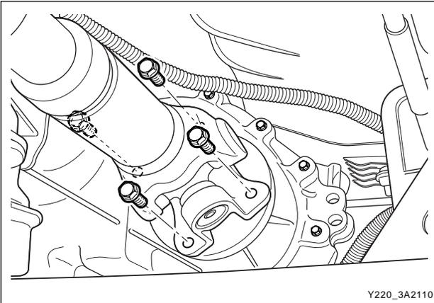
7. Remove the front propeller shaft bolts from transfer case.
