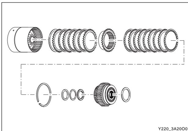
32. Apply petroleum jelly to the No. 5 needle bearing and fit it to the C4 hub.
