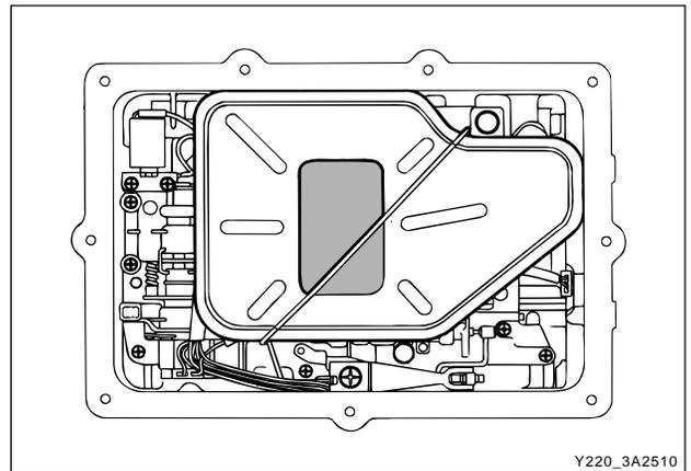
1. Lubricate the oil filter sealing ring with automatic transmission fluid.
