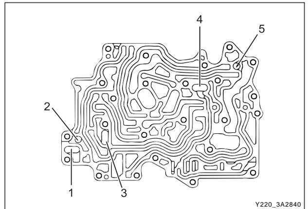
19. Holding the separator plate to the upper valve body to prevent the check balls from falling out, install the upper valve body on the lower valve body. Install all screws finger tight then tighten the screws to specification in the prescribed sequence.
