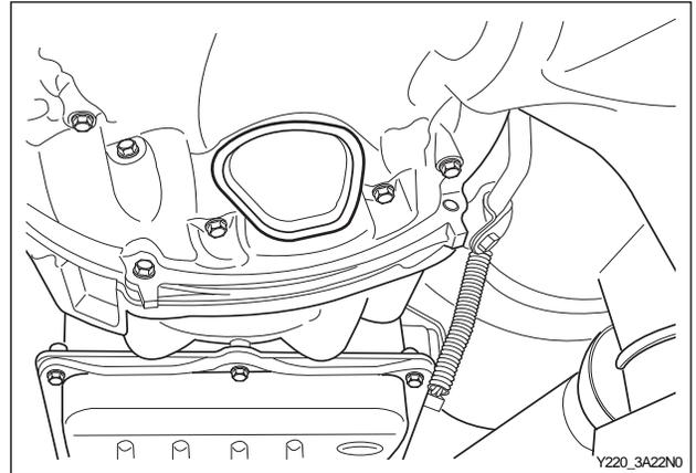
15. Remove the extension housing to case bolts and remove the transmission assembly.
