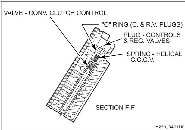
13. Install the converter clutch control valve, spring, plug, and "O" ring.
