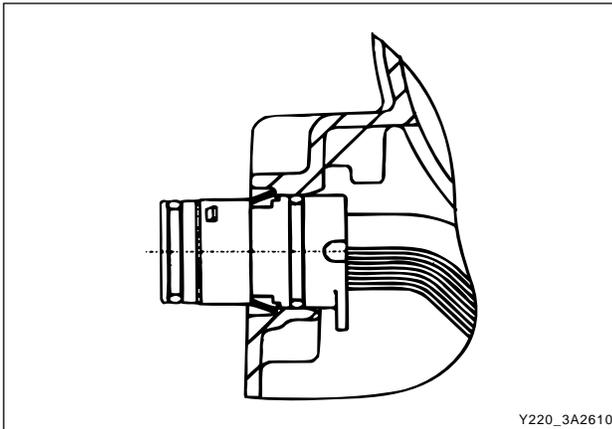
8. Depress the tangs and withdraw the 10 pin connector into the case. Remove the wiring loom assembly.
