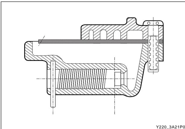
3. Install the line pressure relief valve, tapered end first, spring and disc. Secure with the retaining pin.
