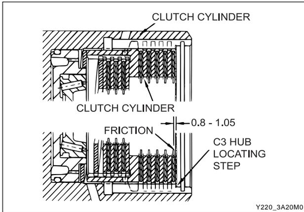
26. Check the clutch pack clearance using only the weight from 0555-336260 clutch pack clearance kit.
