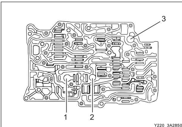
12. Position the third feed ball (large nylon) in the valve body and install the solenoid 6 filter.
