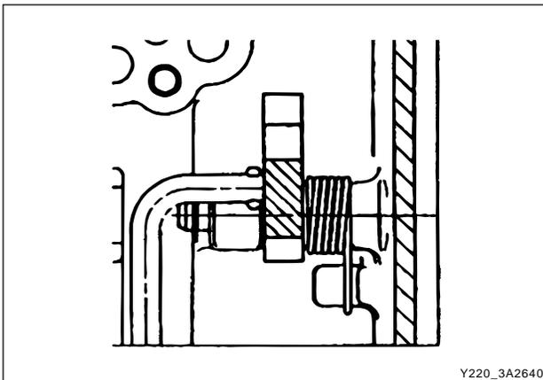
5. Assemble the park rod lever, complete with the return spring and pivot pin, applying a small amount of sealant to the outer end of the pivot pin.
