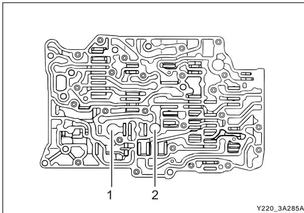
10. Remove the filter (1) and the large nylon check ball (2) from the lower valve body.
