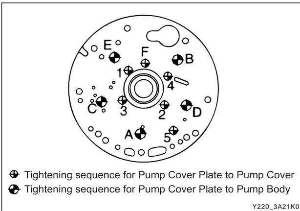
17. Install the cover plate, solenoid 7 with the retainer and the solenoid wiring retainer to the pump cover, ensuring that the periphery of the cover plate is flush with the periphery of the pump cover.
