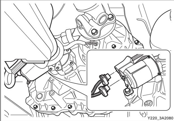
5. Remove the rear propeller shaft bolts.
