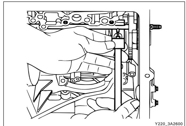
16. Install the new cross shaft seals using cross shaft seal installer 0555-336262 (1) and cross shaft bullet 0555-336263 (2).
