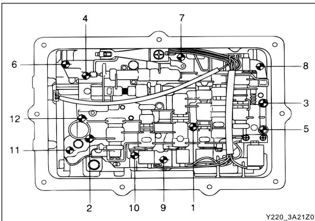
24. Align the valve body assembly on the transmission case and install the manual valve lever to manual valve link. Fit the long end of the link to the manual valve first. Install the securing bolts and tighten to specification in the specified sequence.
