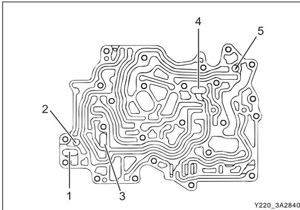
7. Lift the separator plate and gaskets from the upper valve body.
