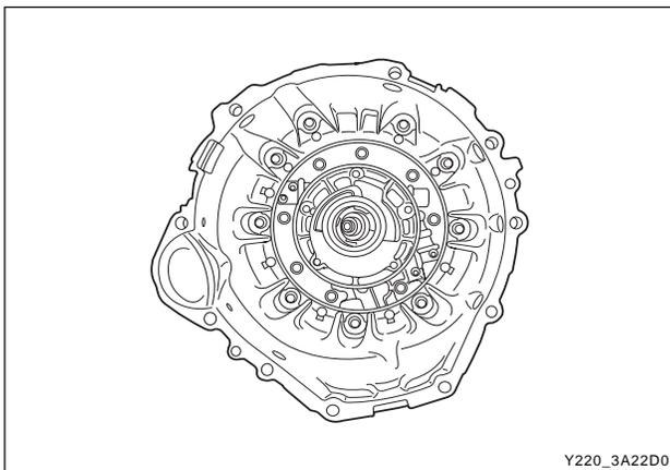
**Torque Converter and Housing Assembly**
