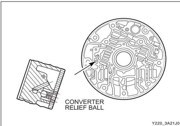
15. Install the converter release check ball and spring.
