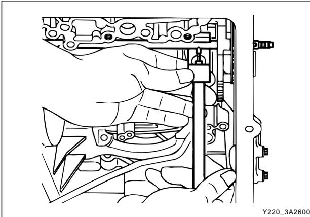
5. Using cross shaft pin remover/installer (detent lever) 0555-336258, press the pin from the cross shaft and withdraw the shaft from the case.
