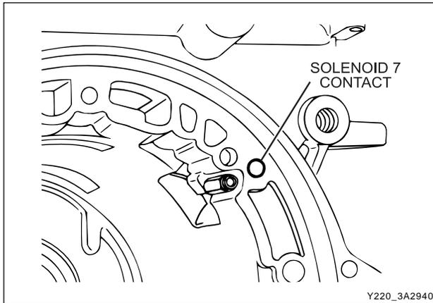
19. Position the wiring loom and locate the solenoid 7 contact and terminal in the pump mounting flange at the front of the case. The solenoid 7 wire is routed under the park rod and cross shaft in the case.
