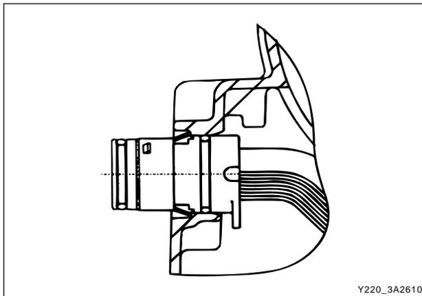
20. Install the 10 pin connector in the case engaging the tangs on the connector in the notches in case.
