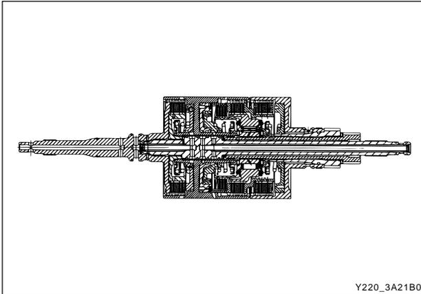
13. Assemble the C1/C2/C4 clutch assembly to the C3 clutch and sun gear assembly.
