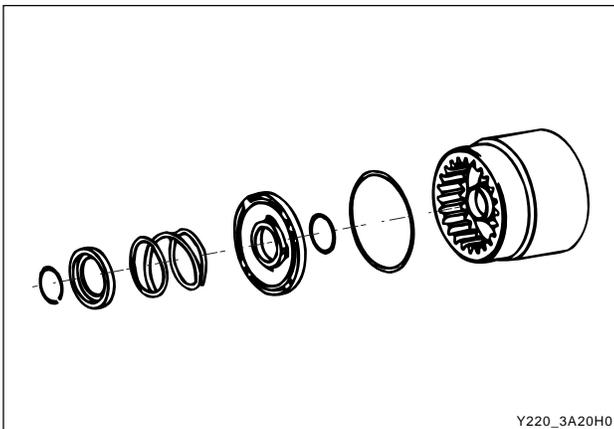
15. Position the cylinder with the C1 cavity upwards. Install the piston into the cylinder until the outer diameter of the piston enters the inner diameter of the cylinder.
