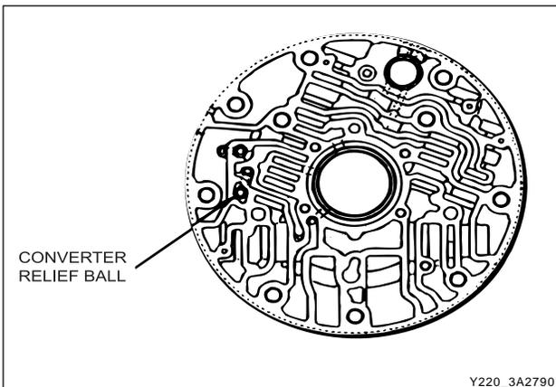
6. Remove the ball check valve and one spring from the pump cover.
