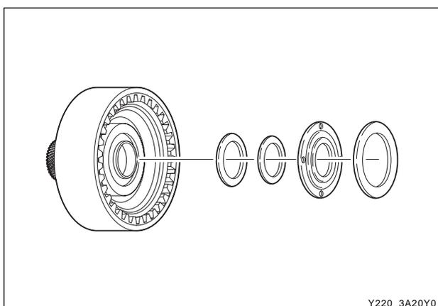
1. Check the overdrive shaft grooves for any defect.
