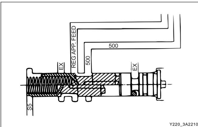
**Converter clutch control valve**
