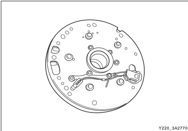
1. Remove the wiring loom retainer plate and remove solenoid 7 with a T30 Torx bit.
