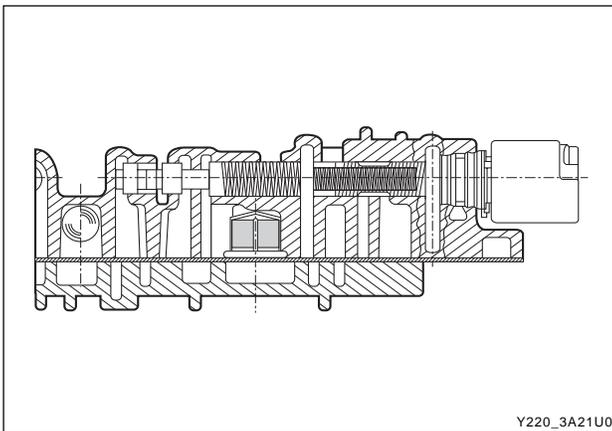
10. Install the solenoid supply valve, spring and retaining plate.
