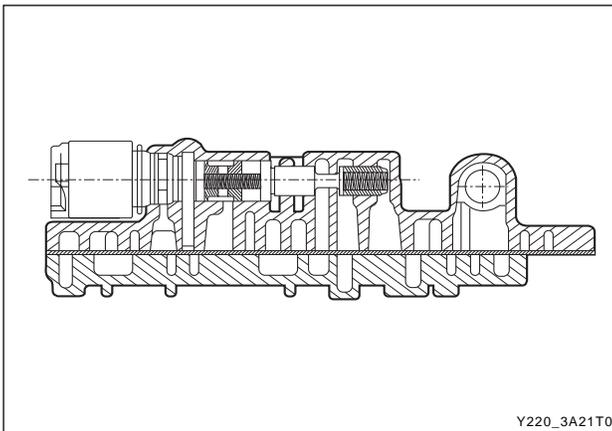
9. Install the Clutch Apply Regulator (CAR) valve, springs, plunger and retaining pin.
