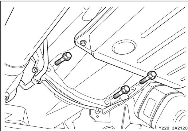
8. Remove the transfer case-to-transmission housing bolts and remove the transfer case.
