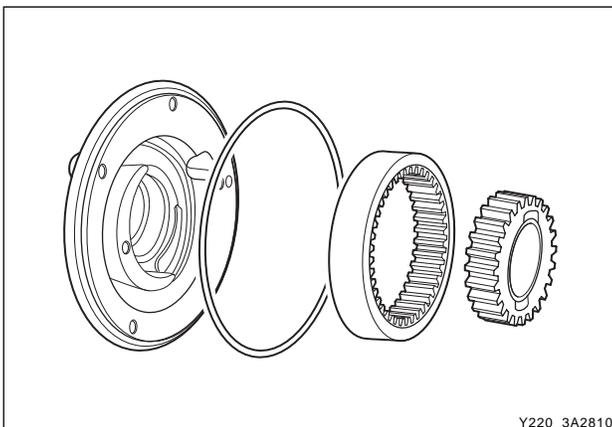
4. Install the pump driven gear and the pump drive gear into the pump body.
