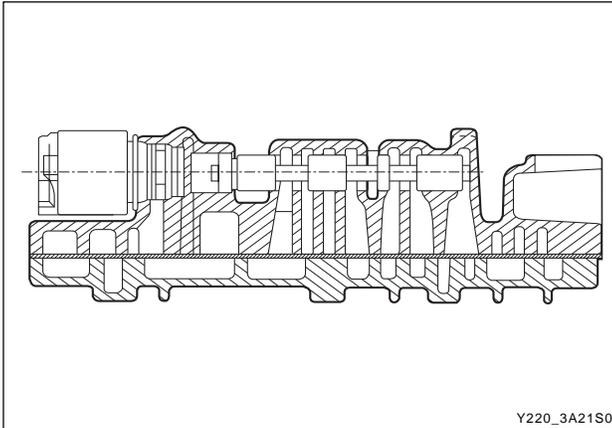
8. Install the 3-4 shift valve and retaining pin.
