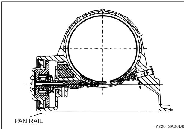
7. Compress the servo cover and fit the servo cover retaining circlip, aligning the gap with the pan rail, and ensuring that it is completely seated in its groove.
