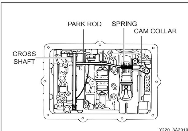
8. Connect the park rod to the manual valve detent lever. Ensure the spring and cam collar is firmly installed on the rod.
