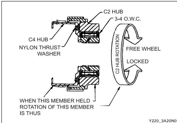
28. Lubricate and fit the 3-4 OWC and end caps to the C2 hub.
