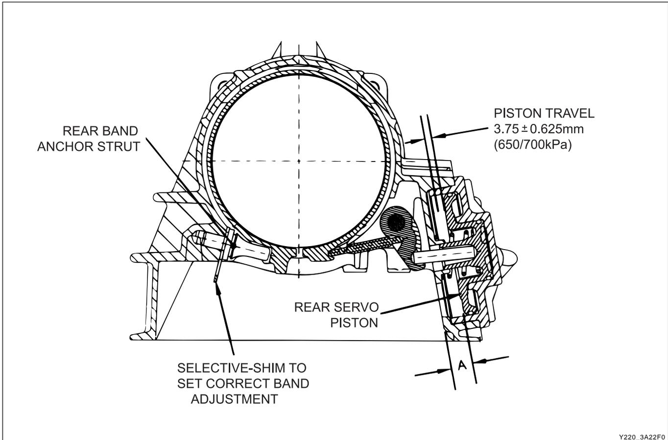
1. Measure distance "A" from the rear servo piston to the inner face of the transmission case using vernier calipers.
