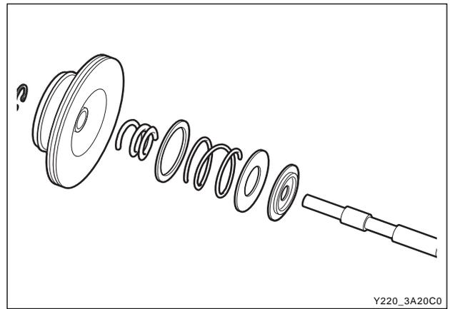
5. Install the front servo block and spring into the case.
