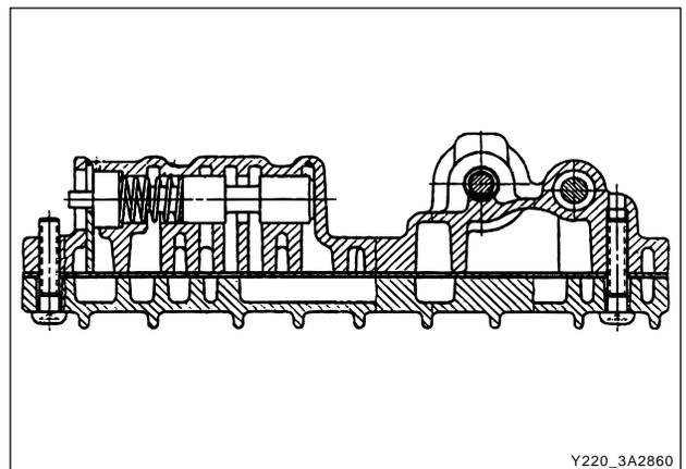
6. Install the 1-2 shift valve, plug and retaining pin.
