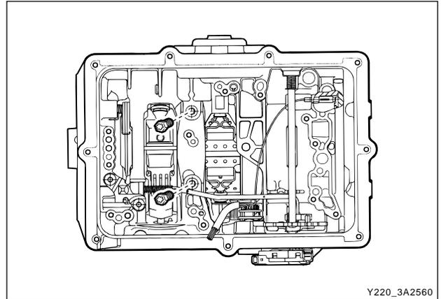
19. Remove the rear band struts and remove the band.
