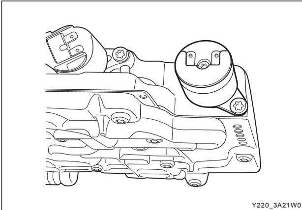
21. Install solenoid 5. Ensure that the solenoid is pushed firmly into the valve body by the retainer and that the screw is tightened to specification.
