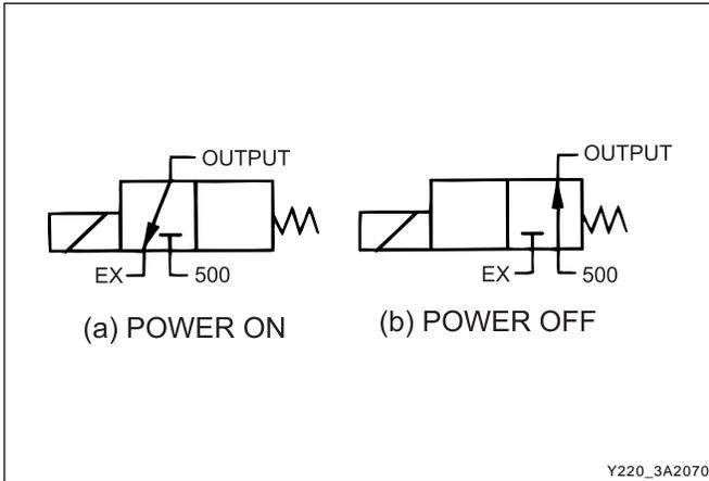
**Variable pressure solenoid multiplexing system**
