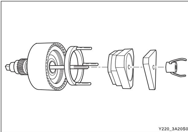
13. Install the circlip.
