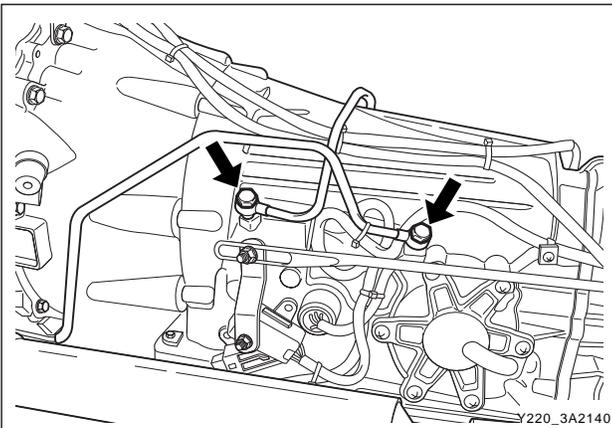
11. Remove the oil cooler pipes.
