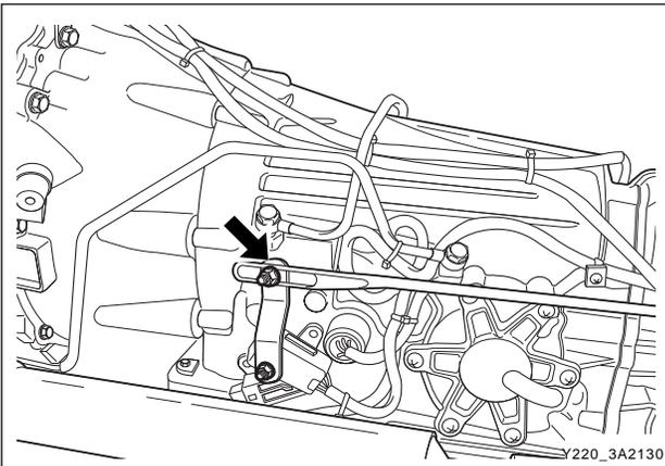
10. Separate the locking clip on shift lever and remove the shift rod.
