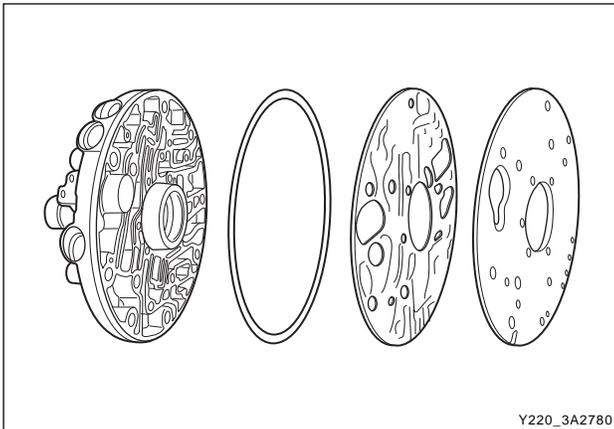
4. Separate the pump body from the pump cover.
