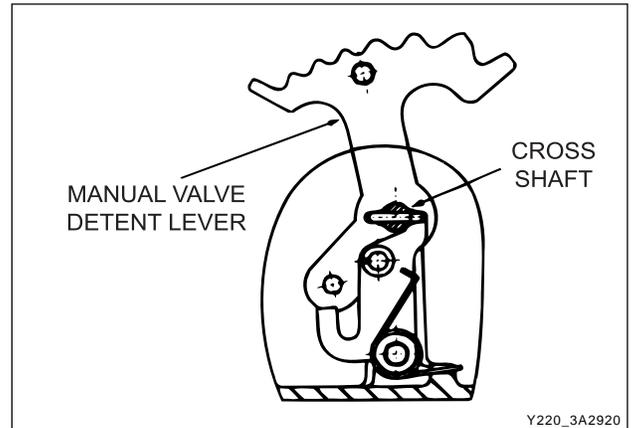
13. Install the detent lever drive pin in the shaft using cross shaft pin remover/installer (detent lever) 0555-336258 with the adaptor over the pin.
