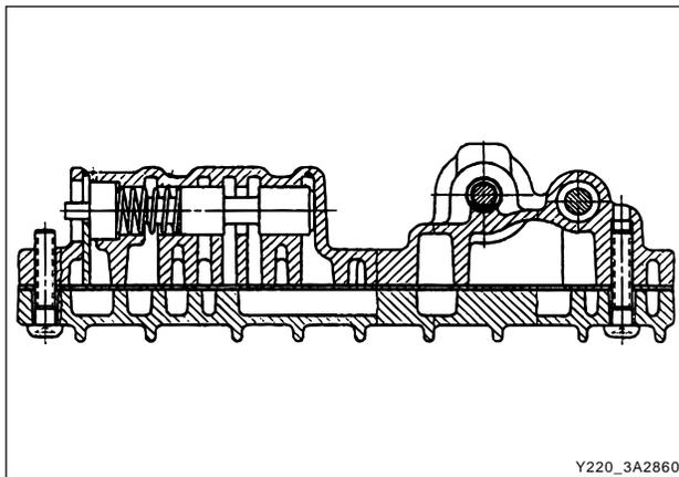
13. Depress the 4-3 sequence valve plug and remove the retaining plate.
