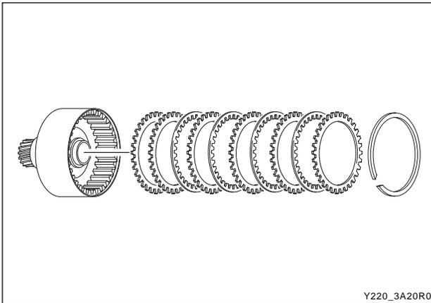
11. Assemble the clutch plates and discs into the cylinder in the following sequence :
