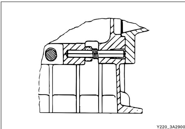
7. Install the parking pawl pivot pin and spring.
