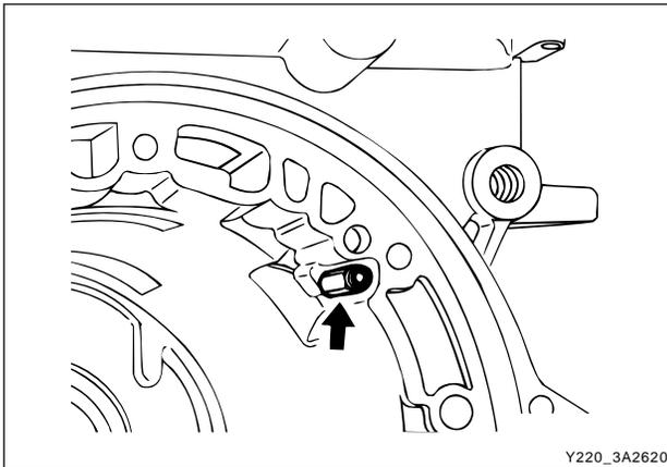
9. Detach the No.7 solenoid wire from the front of the case.
