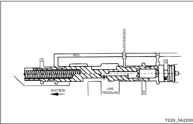
**Converter clutch regulator valve**
