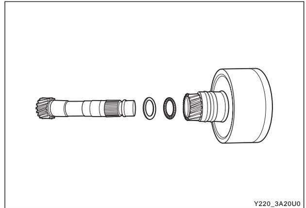
3. Align and fit the C3 clutch assembly over the forward sun gear.
