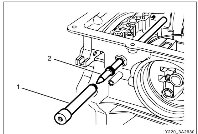
17. Install the inhibitor switch on the case. Torque the bolts as per specifications. Press the pin into the shaft until the tool bottoms using cross shaft pin installer/remover (inhibitor switch) 0555-336265.
