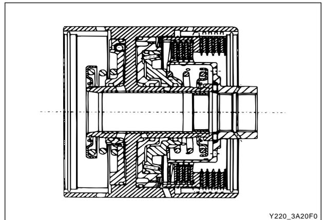
5. Check the C4 piston bleed orifices are clear of obstructions.
