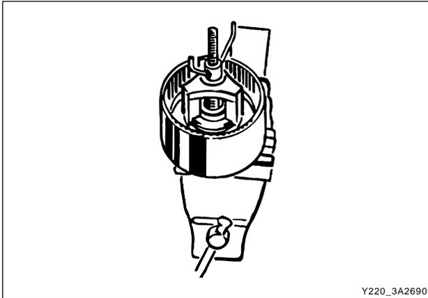
11. Assemble the piston return spring to the piston, and fit the spring retainer over the spring.
