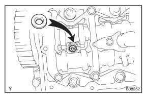
(c) Install a new injection nozzle sheet to the cylinder head.
