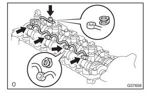
(h) Temporarily install a new gasket and nozzle leakage pipe assy with the 4 hollow screws and union bolt.
