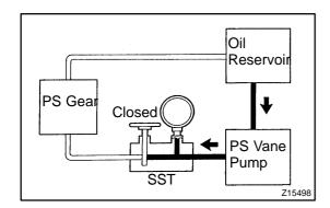
(g) With the engine idling, close the valve of the SST and observe the reading on the SST.
