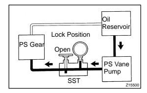
(j) With the engine idling and valve fully opened, turn the steering wheel to full lock.
