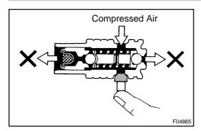
(b) Check the flow control valve for leakage.
