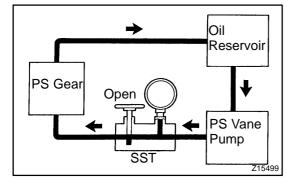
(h) With the engine idling, open the valve fully.
