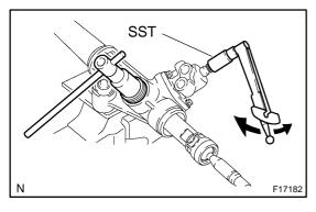
(f) Using SST and a torque wrench, tighten the cap until the preload is within specification.
