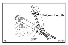
ing SST, torque the rack end. SST 09922-10010
