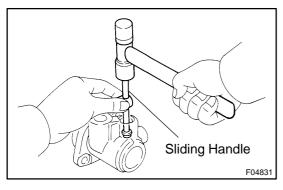
(b) Using plastic hammer and sliding handle, lightly tap in a new union seat.
