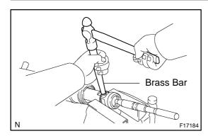
(c) Using a brass bar and hammer, stake the washer.
