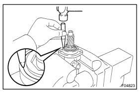
(f) Using a punch, stake the nut.
