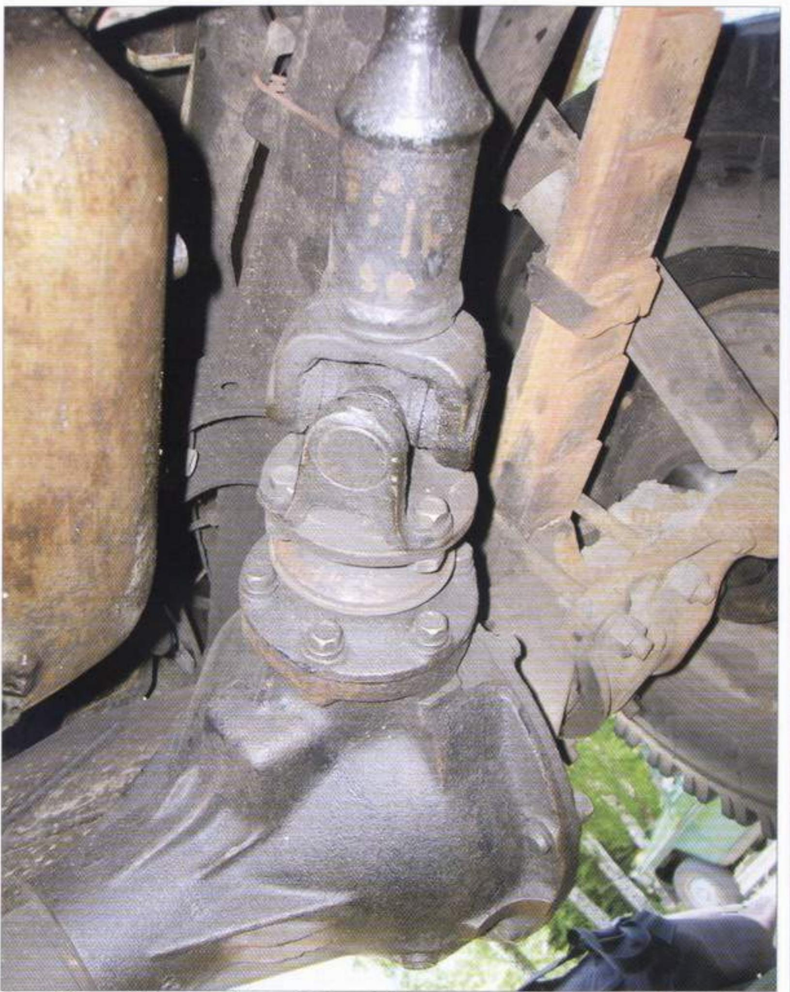
Front differential gear casing and drive shaft. Lower part of the engine and gear-box •
