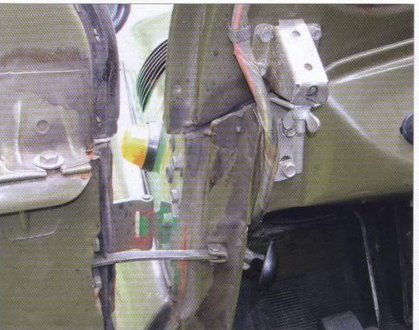
Close-up of the inner side of the door, hinges and handles.
