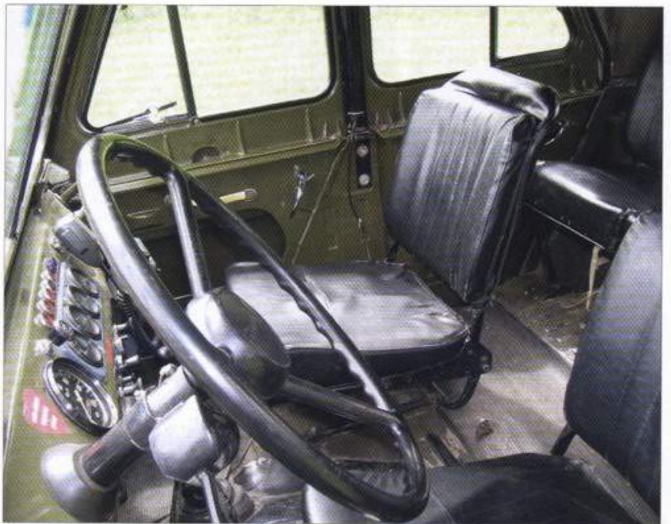
Details of driver's seat, the standard three-spoke steering wheel and column. Metal made dashboard with instrument panel. The vehicle controls are similar to the civil vehicle with manual gearbox, but include some military features like standard light and ignition switches. The direction indicators switch
