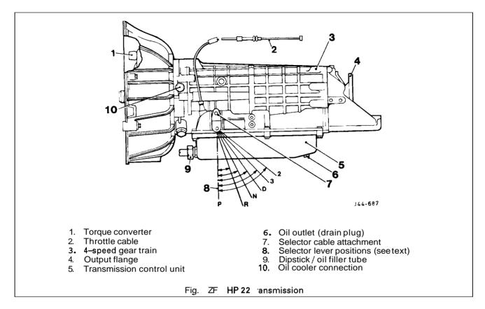
The transmission provides six gearshift positions:
