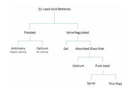
The modern OE battery is the flooded calcium, maintenance-free battery. This is not a Valve Regulated battery. The terms "Valve Regulated" and "Valve-Regulated Lead Acid (VRLA)" are reserved for the SLI batteries that allow for any gas generated by the charging process (hydrogen and oxygen) to be recombined inside the battery back to water. This negates the need for adding any water during the life of the battery.
