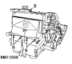
8. Remove 5 screws securing casings.
