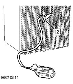
12. Remove evaporator thermistor.
