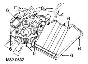
**6.** Remove 6 screws and 4 clips securing main casing and remove top half of casing.
