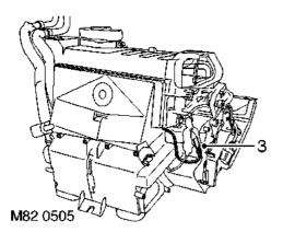
**3.** Disconnect multiplug from evaporator thermistor.
