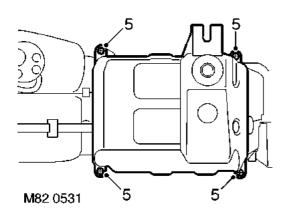
5. Remove 4 screws securing lower part of casing, release and remove lower casing.
