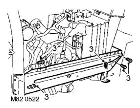
**3.** Remove 5 bolts securing seat support bracket and remove bracket.
