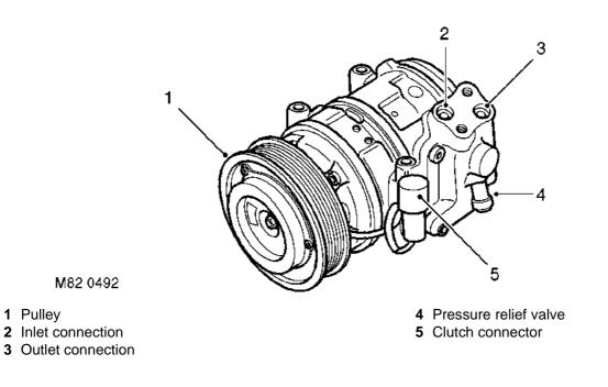
The compressor circulates the refrigerant around the system by compressing low pressure, low temperature vapour from the evaporator and discharging the resultant high pressure, high temperature vapour to the condenser.
