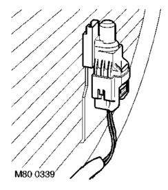
2. Release ambient air temperature sensor from support bracket, disconnect multiplug and remove sensor.
