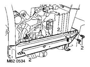
2. Remove 5 bolts securing third row seat support bracket and remove bracket.
