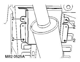
2. V8 models: Remove 4 clips securing rear exhaust heat shield and remove heat shield.
