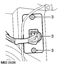
**3.** Remove 2 screws securing resistor pack to casing. Remove resistor from casing.
