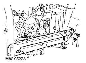
**6.** Remove 5 bolts securing seat support bracket and remove bracket.
