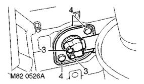
**3.** Remove 2 bolts securing high and low pressure pipes, release pipes and discard 'O' rings.
