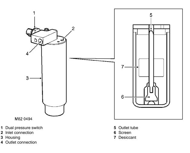
The receiver drier removes moisture and solid impurities from the refrigerant and also acts as a refrigerant reservoir.
