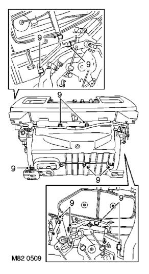
9. Remove 12 spring clips securing casings.
