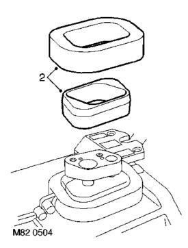
2. Remove bulkhead and evaporator pipe seals.
