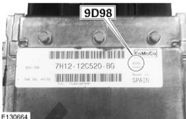
Remove the engine cover, reference GTR 501-05 interior trim, using a mirror to read the 4/5 digit number on the top right corner of the PCM. Note the batch code reference number and identify the build date of the PCM (see graphic E130664). If the build date is earlier than 14th October 2009, replace the powertrain control module reference GTR 303-00 and continue to step 7.
