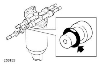
5. Withdraw the air bleed valve from inside the brass fitting. Inspect the O-ring and plastic body for splits and damage.
